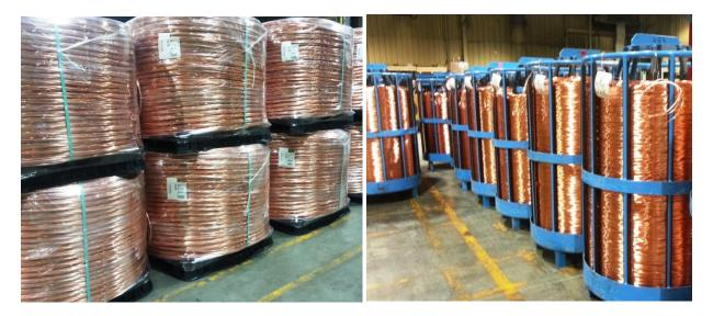
Figure 1. Copper Rod (left) and Copper Wire (right) Made at Essex
